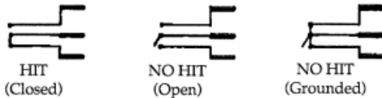
Fig. 10 EPEE HIT REGISTRATION (SCHEMATIC)
