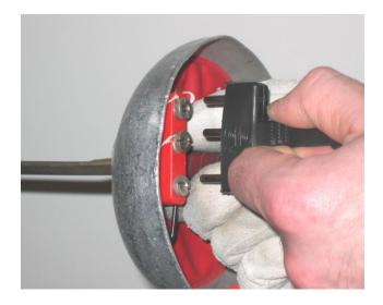
8. Insert the plug and slide the retaining clip over the plug.
