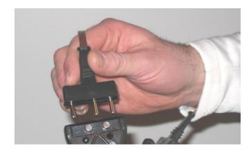
4. Fit the retaining clip to secure the plug-in place.
