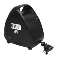
F.I.E regulation spool compatible with any recorder. Moulded fibre glass case, self colour with integral handle. Triple core cable, plastic covered with Kevlar strain cord reinforcement. Stainless steel commutator with silver studs gives perfect contact at all times. Every part is replaceable from our price list and the complete spool can be taken apart or assembled in under 30 seconds without using any tools.
