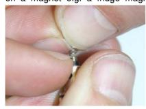
keeping a finger over the point so that it does not spring off when you remove the second screw! The screws are very easy to lose so this is best done on a clean table. Inside the tip are two springs, the first is a small
