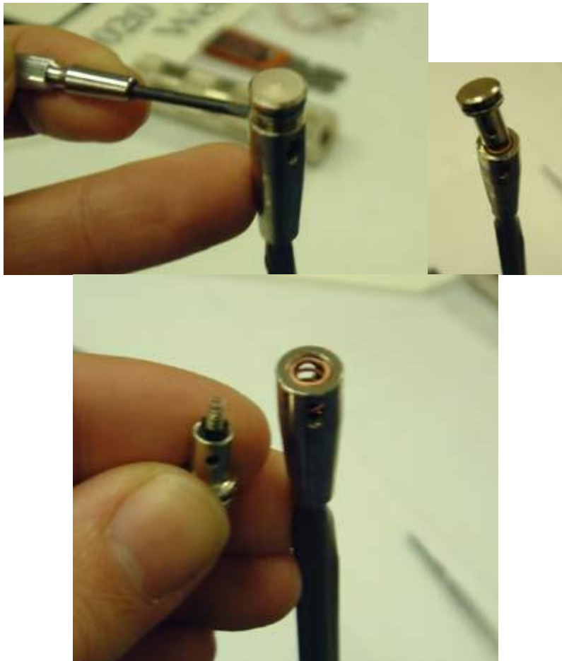
These are the parts found in an epee point.
